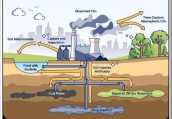
Geological sequestration: Once CO2 has been captured using CCUS technology, it's pressurised and turned into a liquid-like form known as 'supercritical CO2'. From there it's transported via pipeline and injected into the rocks found in the formations deep below the earth's surface. This is a process called geological sequestration.
