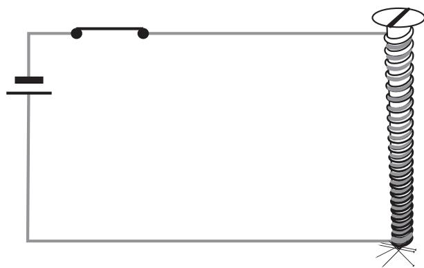
**Fig. 14.19** An electromagnet
