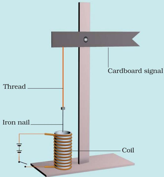
**Fig. 14.26** A working model of a railway signal
