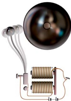
**Fig. 14. 20** Circuit of an electric bell
