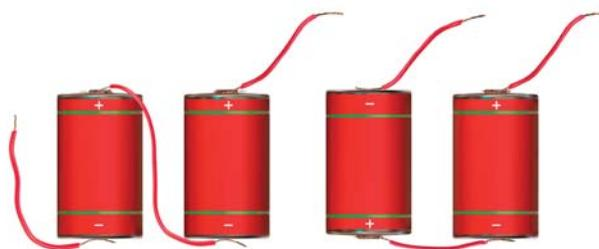
**Fig. 14.3** Connecting two cells together to make a battery
