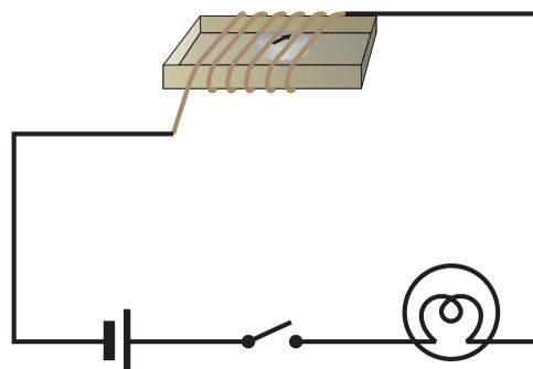
**Fig. 14.17** Effect of current on a compass needle
