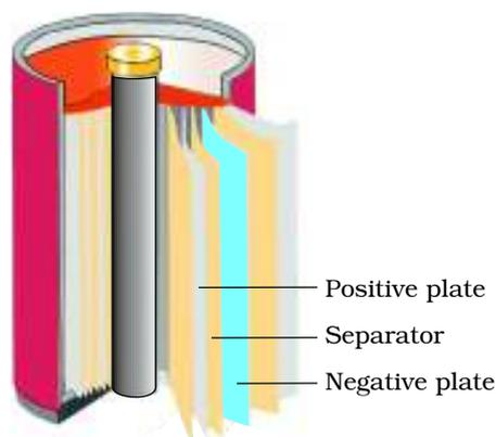
Another important secondary cell is the nickel-cadmium cell (Fig. 3.11) which has longer life than the lead storage cell but more expensive to manufacture. We shall not go into details of working of the cell and the electrode reactions during charging and discharging. The overall reaction during discharge is:
